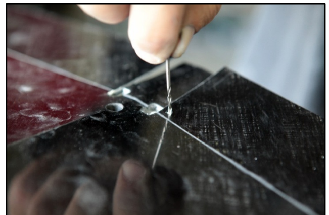
Figure 2.17 - Holes for gluing horn in flaperon
