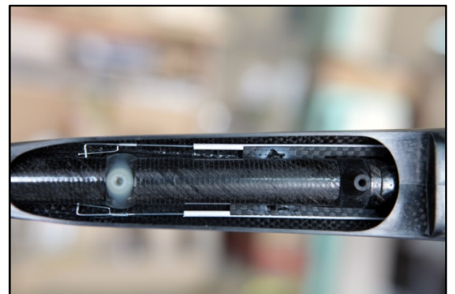
Figure 2.39 - Fixing the aileron linkage inside the fairing
