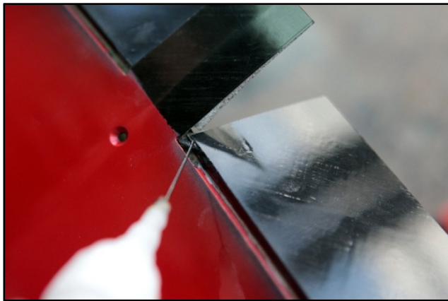
Figure 2.21 - Bonding horn inside the aileron
